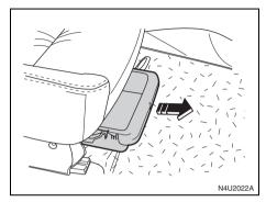
Your vehicle may have a sliding storage tray located under the front passenger seat. To use the tray, pull up on the end of the tray and pull it toward the instrument panel. Push the tray toward the seat to return it to its original position.
